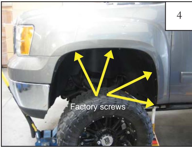
Using a 7mm socket, remove four factory screws from wheel well and save for reinstallation.
