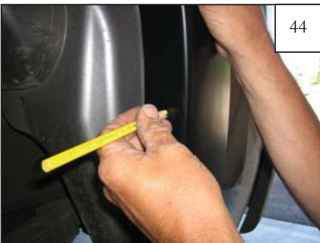
Holding flare in position on fender, use a grease pencil to mark eight hole locations.
