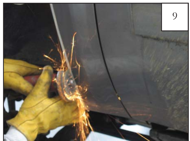
Cut along the outside of fender to 18'' mark. See picture in step 10.
