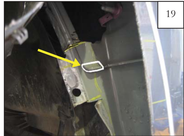
Cut off outlined tab to make bend in the next step easier.
