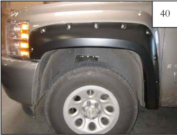
Reinstall wheel. Completed front flare installation.
