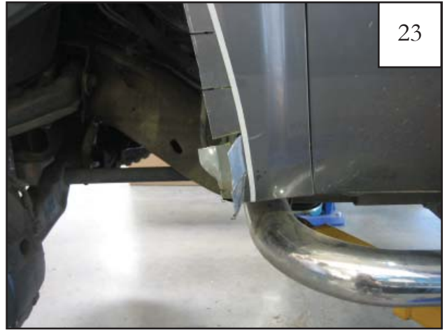
Bend lowest two metal tabs outward.
