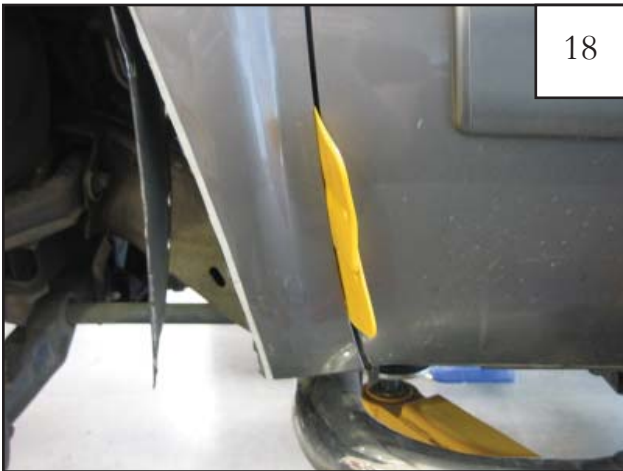
To prevent paint damage, insert plastic spacer between fender and door. This will keep the fender from hitting the door edge while pounding back sheet metal in the next few steps.
