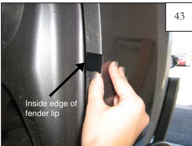
Center a supplied Tab (MT1-0002) over the marks made in step 41, aligning edge of tab with inside edge of fender lip (tab may extend over outside of fender).
