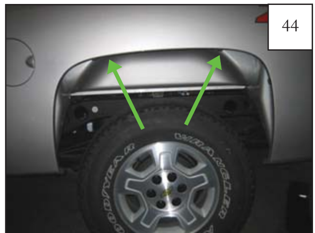
Slide a supplied Clip (CL1-0022) over top two tabs. Clips may need to be adjusted to align with holes in flare.
