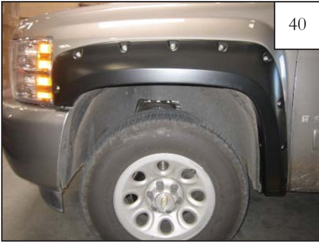
Reinstall wheel. Completed front flare installation.
