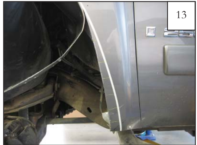
Bend inner fender metal away from fender.
