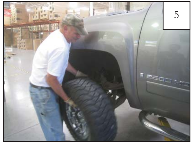
Support vehicle and remove tire.
