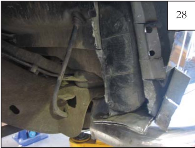
Cut pinch seam at mark made in previous step. Bend flange back even with firewall.
