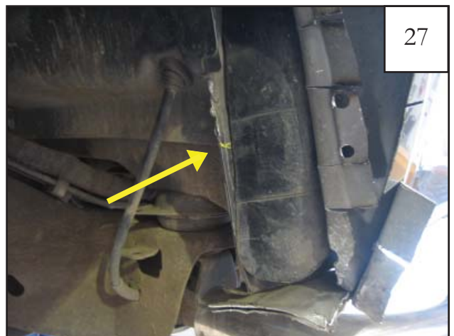
Mark inner pinch seam at location shown.
