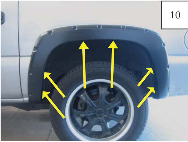
Tighten the topmost two Screws first, then the forward two, and then the rearward two.
