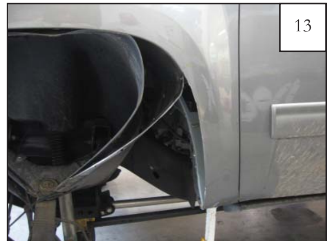
Bend inner fender metal away from fender.
