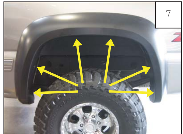
Install six tuflocks using a #2 stubby screwdriver.
