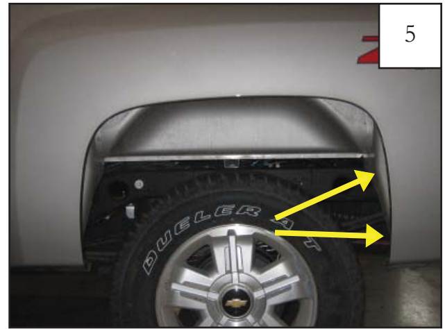
Remove two factory screws with a #2 stubby screwdriver.
