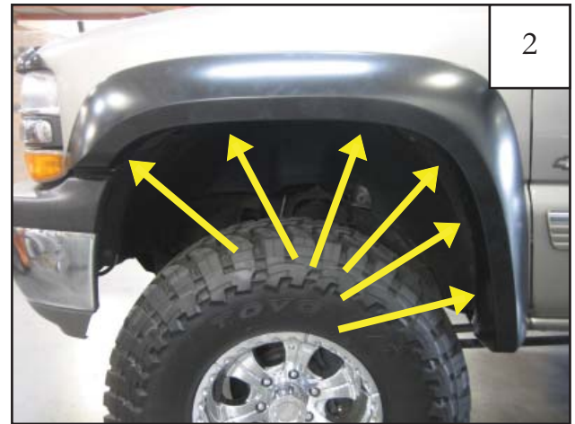
Install six tuflocks using a #2 stubby screwdriver.
