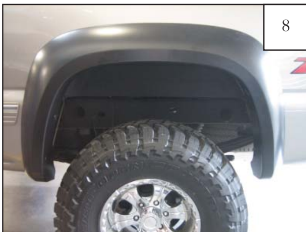
Completed rear flare installation.
