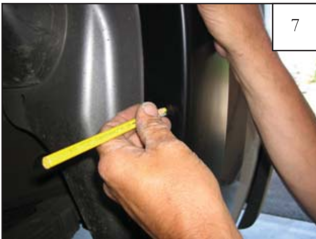
Holding flare in position on fender, use a grease pencil to mark the five clip locations.
