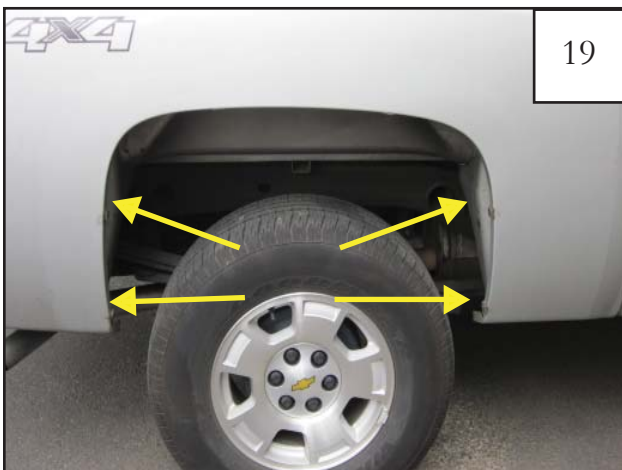
Slide a supplied Clip (CL1-0005) over lower four tabs. Clips may need to be adjusted to align with holes in flare.
