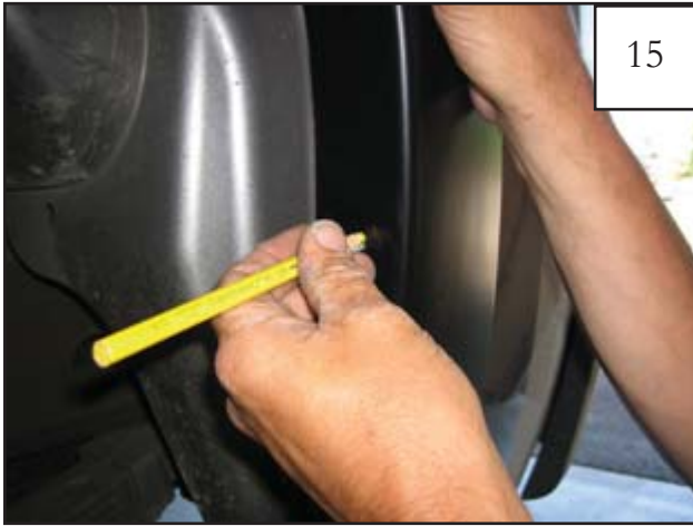
Holding flare in position on fender, use a grease pencil to mark the four clip locations.
