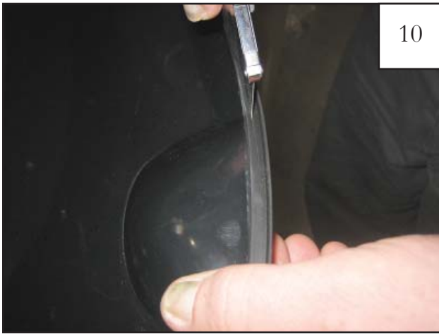
For the Rear Driver's side with gas door cut out only: In the area of the cut out, use a knife to trim the backside of the edge trim at the center as shown.
