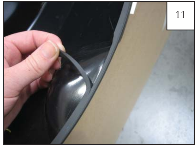
Carefully peel cut portion of edge trim and discard. This will prevent the edge trim from interfering with the gas door.
