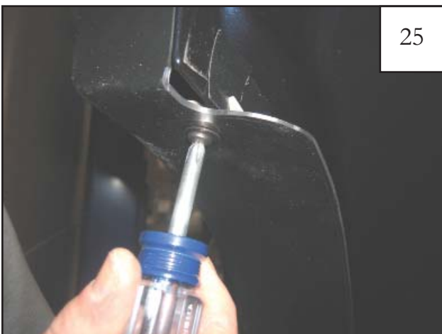
Replace the Door Piece on the door, aligning holes in door piece with holes in Clips. Start four Screw/Washer assemblies but do not tighten .
