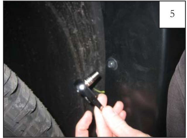
Holding flare in position on fender, reinstall factory screws removed in Step 4. If necessary, use awl (or similar pointed tool) to locate holes.
