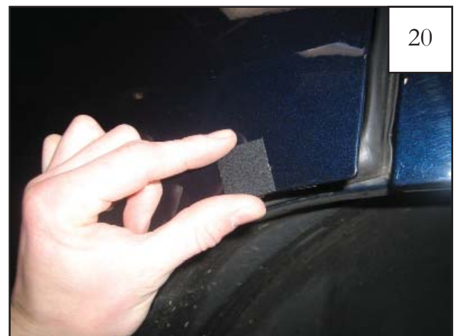
Apply corresponding Tabs (MT1-0001) on the outside of the door, aligning with Tabs applied in Step 19.
