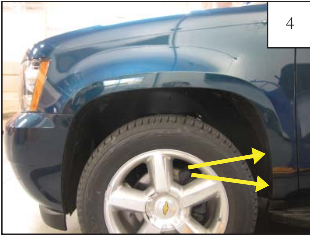
Using a 7mm socket, remove two factory screws. Retain screws for later use.
