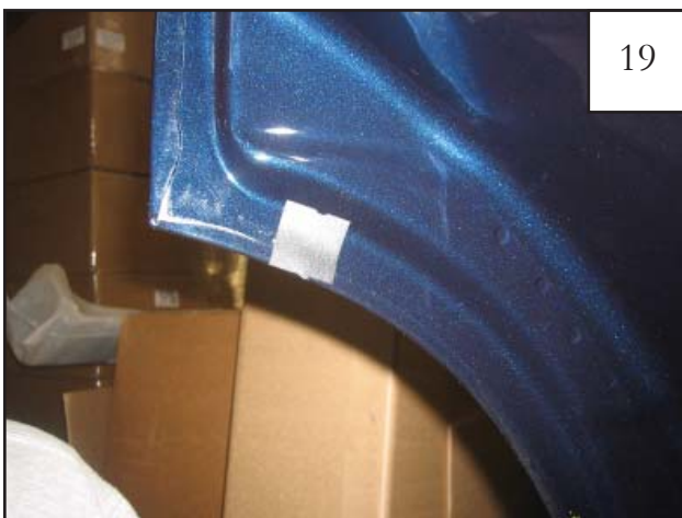
Apply a supplied Tab (MT1-0001) to the inside of the door, centering tabs over the marks made in Step 18 (4 places).
