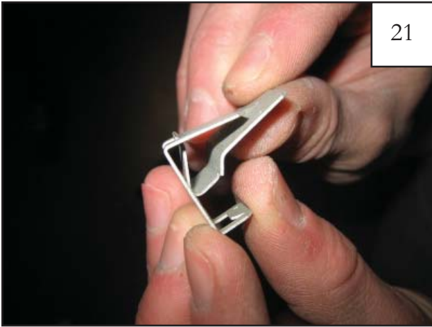
Slide Clip (CL1-0008) into Clip (CL1-0010) as shown. Do not snap clips shut.
