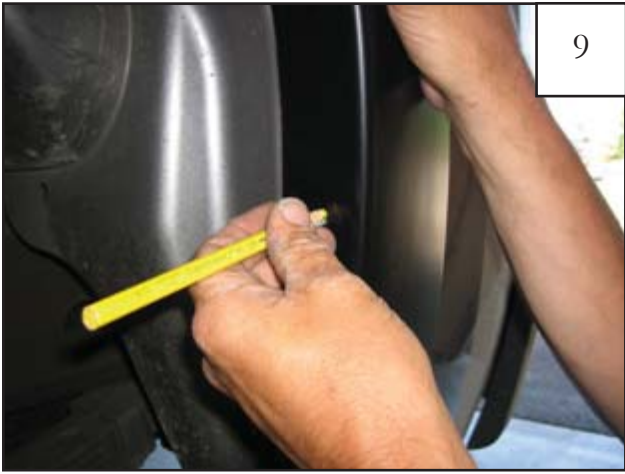
Holding flare in position on fender, use a grease pencil to mark eight hole locations.
