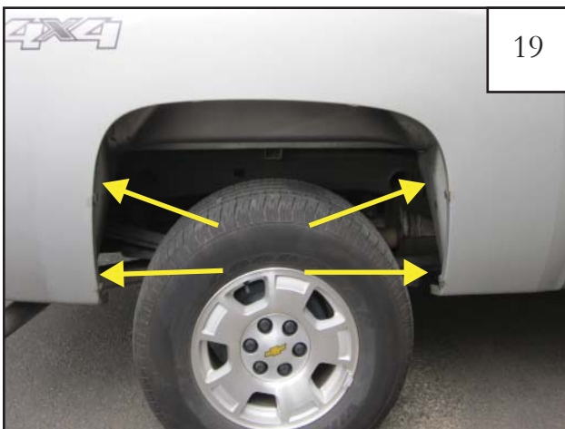
Slide a supplied Clip (CL1-0005) over lower four tabs. Clips may need to be adjusted to align with holes in flare.
