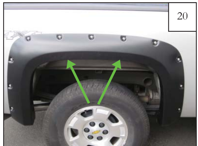
Reposition flare on fender. Start a supplied Screw (SW1-0058) through upper two hole locations and through each Clip (CL1-0022) installed in step 17. If needed, use awl to locate holes.
