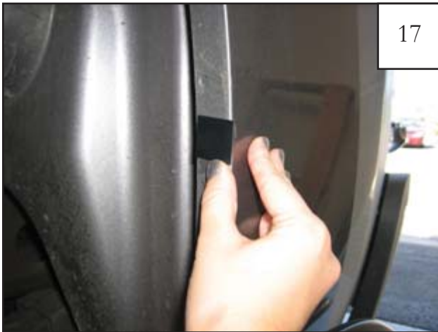
Center a supplied Tab (MT1-0002) over the marks made in step 15, aligning edge of tab with inside edge of fender lip (tab may extend over outside of fender).
