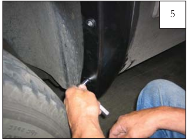
Position flare on fender and reinstall the four factory screws removed in Step 4.
