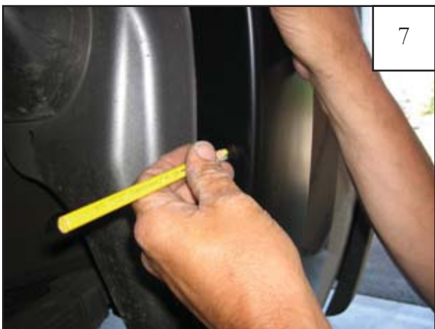
Holding flare in position on fender, use a grease pencil to mark seven hole locations.
