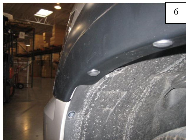
Install a supplied Plastic Tuf-lok through forward hole in flare.
