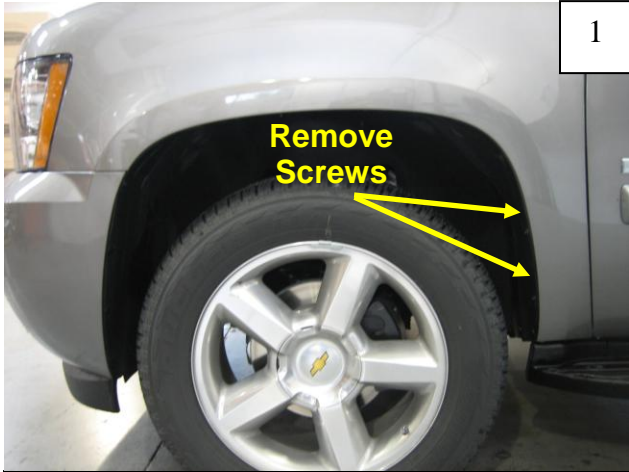
Using a 9/32" socket, remove two factory screws. Retain screws for later use.
