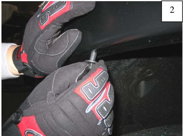
Holding flare in position on fender, install two supplied Plastic Tuf-loks.
