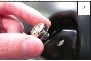
Put each Bolt/Washer combination through a pocket hole in the flare, Bolt head and Washer on the outside.
