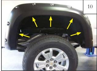
Holding flare in position, start five supplied screws (SW1-0056) starting through the top center hole working outward. Use awl to align clip with mounting hole.
