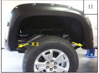
Start three supplied screws (SW1-0056) into one forward and two rearward mounting holes. Fully tighten all screws.
