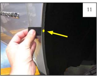
Wrap one supplied tab (MT1-0034) around inner lip of sheet metal over the marked location.
