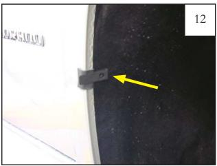
Once tab has been applied, install one clip (CL1-0009) over tab.
