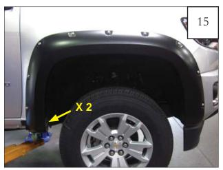
Start two supplied screws (SW1-0056) into the two botton rear mounting locations. Fully tighten all screws.
