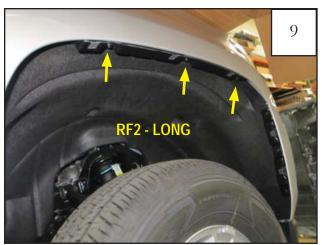
Install the long mounting bracket (RF2) into top of wheel well, using three factory fasteners and a T-15 torx bit. Tighten screws.
