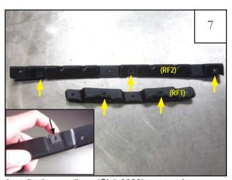
Install three clips (CL1-0028) onto the upper mounting bracket (RF2) and two clips (CL1-0028) onto the front mounting bracket (RF1). Repeat same step for driver side brackets (LF1, LF2).
