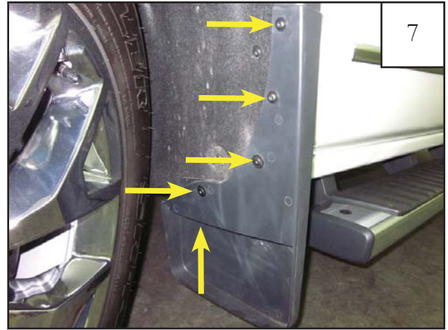
FOR MODELS WITH FACTORY MUDFLAP: Remove mud flap fasteners. Use T-30 Torx bit for two upper fasteners. Use T-15 Torx Bit for two lower fasteners and use a Phillips Head Screwdriver for Bottom fastener.
