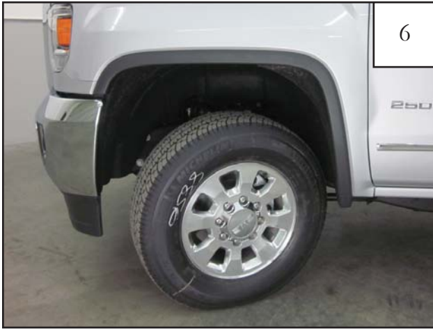
Turn front tire outward for easier installation. Factory wheel arch molding must be removed prior to part installation. See next steps.
