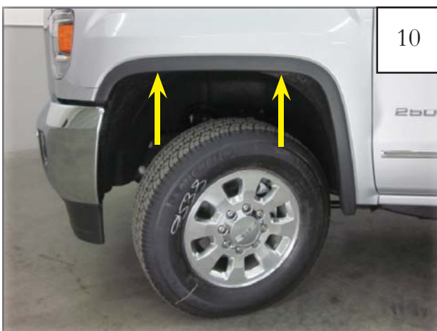
Remove two fasteners along top of factory wheel arch molding using a T-15 Torx bit.
