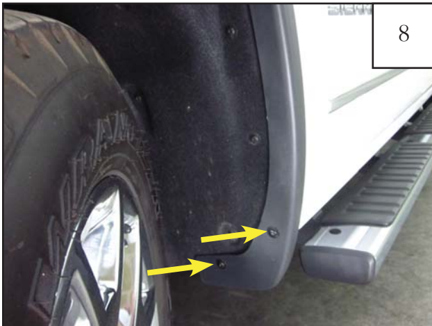
Remove two lower fasteners from factory wheel arch molding using a T-15 Torx Bit.
