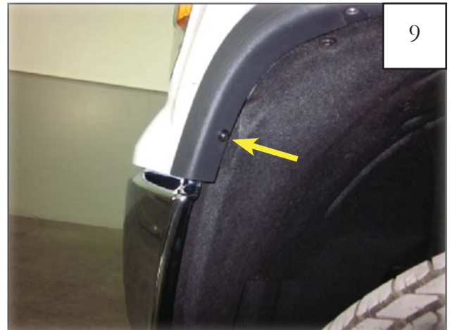
Remove fastener from front of factory wheel arch molding using a 9/16" socket and wrench. Save for reinstallation.
