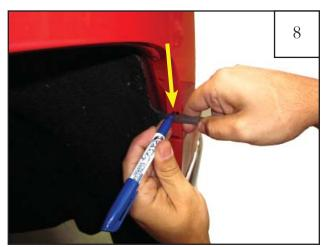
Remove the flare. At the marked locations made in Step 6, measure inward 22mm from the edge of the fender and mark with grease pencil or marker. These are the marks to be drilled.
