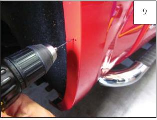
Using a 3/32" drill bit, drill pilot holes at the marks made in Step 8.
