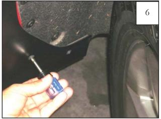
Hold flare in place and start supplied Screw (SW1-0056) through two bottom rear holes in flare and into factory holes in rear of wheel well. *Do not tighten.*
