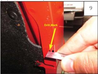
Remove the flare. Using the marks made in step 7 as a guide, measure inward from the outside edge of the fender to verify proper depth of original marked location. Mark must be minium of 10mm in from outside edge of fender, if short, adjust mark to 10mm.
