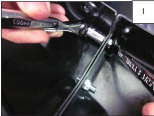
**FOR 2014-2015 SILVERADO 1500 MODELS ONLY:** Insert the Screw/Nut assembly (SW1-0005/ NU1-0001) through the hole drilled in the end of the Front Main Flare and into the corresponding hole in the Front Bumper Piece. Two places and tighten.
