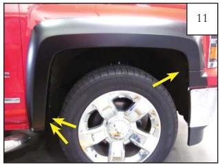
Locate flare into position on vehicle. Re-install supplied screw (SW1-0056) through two bottom rear holes in flare and into factory hole in front of wheel well.
