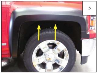
To mount the flare into position, hold the flare 2-3" inches below the top lip of the wheel well. Push in and slide up to allow the flare the fully seat against the wheel well opening.
