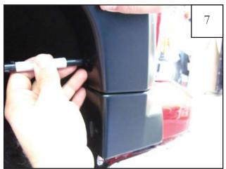
While holding the flare firmly in position, mark the remaining five hole locations with a grease pencil or sharpie. Using the holes in the flare as a guide. Press inward firmly on the flare above each hole location before marking each mark, this will ensure proper fit. See next step.
