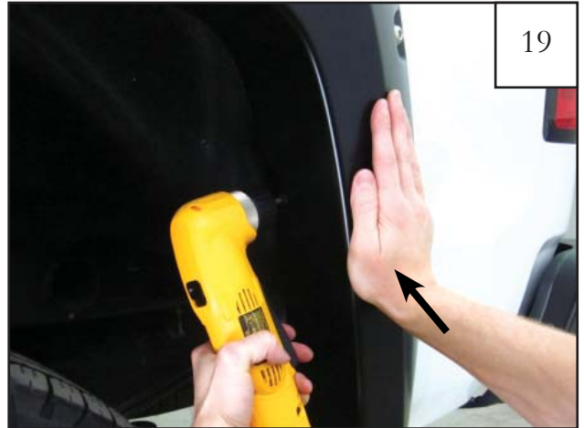
Install self-tapping screws (SW1-0015) into pilot holes drilled in step 36 (3 places). Press flare firmly towards the vehicle while fully tightening.
