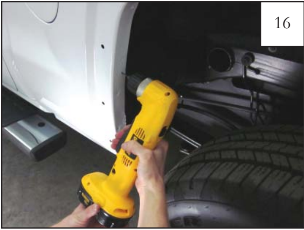
Using a 3/32" drill bit, drill pilot holes through sheet metal at the marks made in Step 34.
