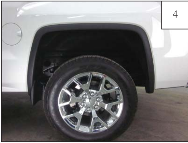
Factory wheel arch molding must be removed prior to part installation. See next steps.
