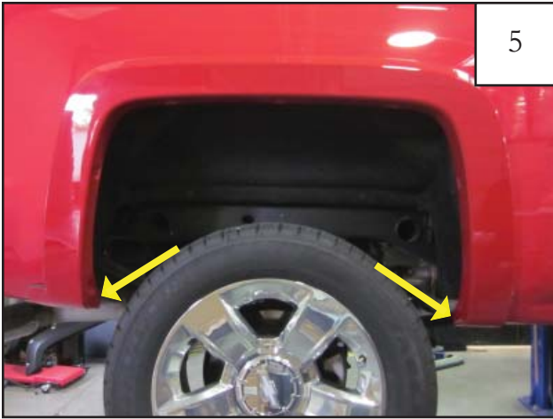
5 Hold flare firmly in place on fender. Start supplied screw (SW1-0056) at bottom most screw locations (shown). Do not tighten.
