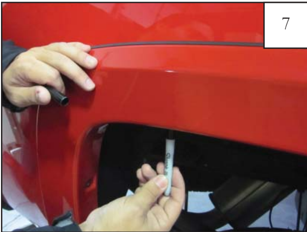
7 Using a grease pencil, mark five locations using the holes in the flare as a guide.
