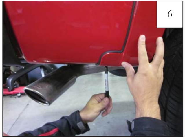
6 Using a grease pencil, mark the rear bottom fastener using the flare as a guide.
