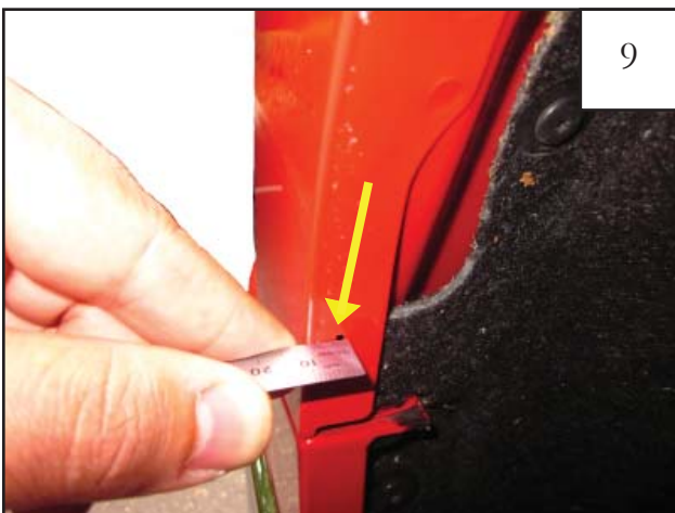
9 Remove the flare. At the marked locations made in Step 7, measure inward 22mm from the edge of the fender. These are the marks to be drilled.
