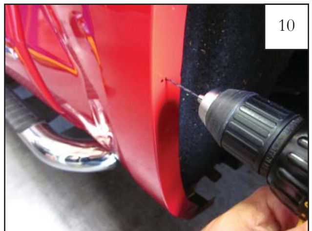
10 Using a 3/32" drill bit, drill pilot holes at the marks made in Step 9.
