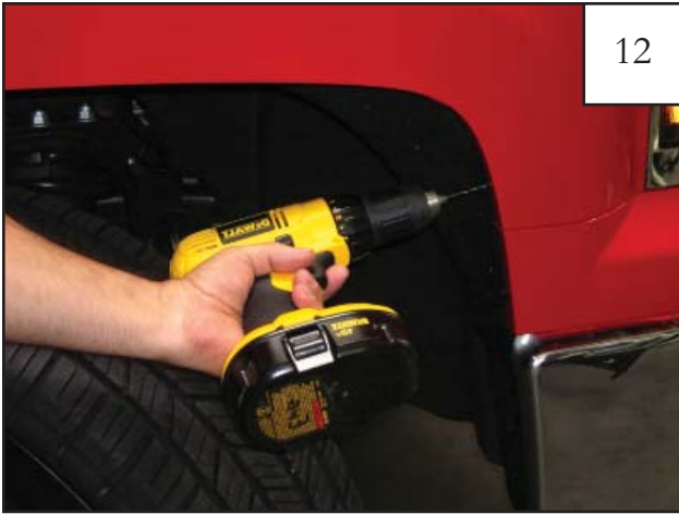
Using a 3/32" drill bit, drill pilot holes at the marks made in Step 11.
