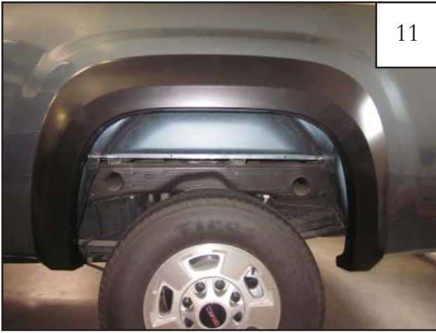
Completed rear flare installation.
