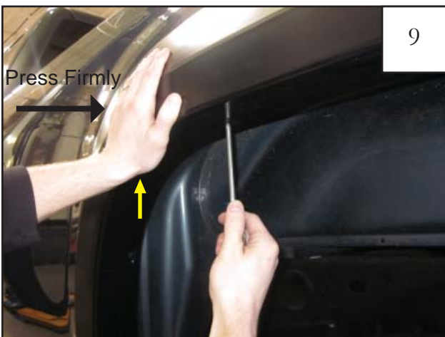
Reposition flare on fender. Check that flare is positioned correctly around wheel well. If not, adjust before tightening screws. Start a supplied screw (SW1-0058) through the two uppermost holes in the flare and into each clip installed in Step 2. Firmly press the flare up and toward the vehicle while tightening both screws.
