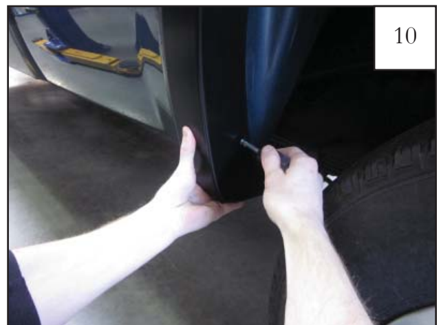
Start a supplied Screw (SW1-0050) through each of the remaining holes and into each Clip installed in Step 8. If needed, use scratch awl (or similar pointed tool) to locate holes. Tighten all screws.
