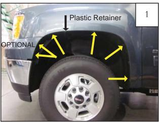
Remove factory mudflap if applicable. Using a 7mm socket, remove four factory screws from wheel well and save for reinstallation. If installing optional bumper piece, remove two front factory screws from bumper and save for reinstallation. Note: Some models have plastic retainers at top center; remove with pry tool and discard if on vehicle.
