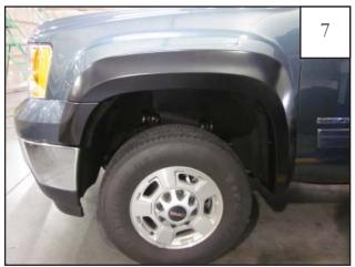
**OPTIONAL BUMPER PIECE:** Completed front flare installation.
