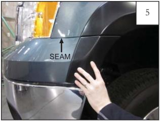
Position flare on fender, aligning bumper piece and flare seams with factory seam. Using a 7mm socket, reinstall factory screws removed in step 1. If needed, use a scratch awl (or similar pointed tool) to locate holes. **DO NOT FULLY TIGHTEN SCREWS**
