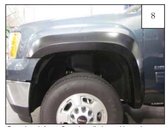
Completed front flare installation without bumper piece.
