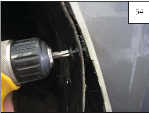
Starting with the top location, fasten inner fender metal to bent tabs of outer fender with Screws (SW1-0056) through holes drilled in last step (4 locations).
