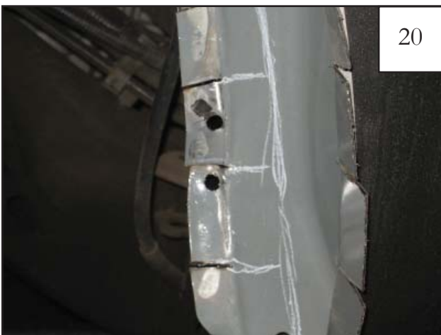
Using outer edge as a guide mark along flange parallel with the inner wall. Mark flange to extend cut lines to line parallel with the inner wall.
