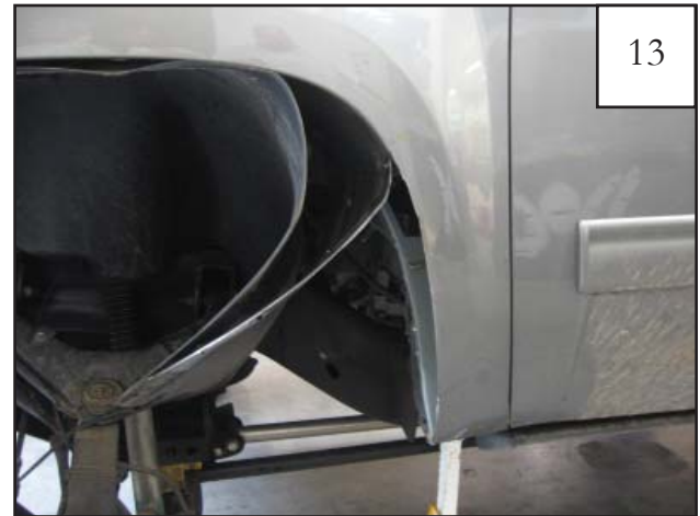
Bend inner fender metal away from fender.
