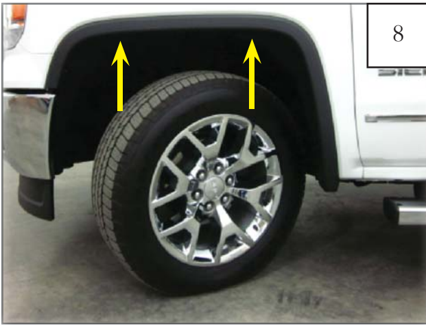
Remove two fasteners along top of factory wheel arch molding using a T-15 Torx bit.
