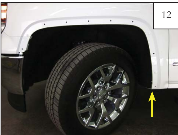
Reinstall factory fastener removed in step 9 using a 1/2" socket and wrench.
