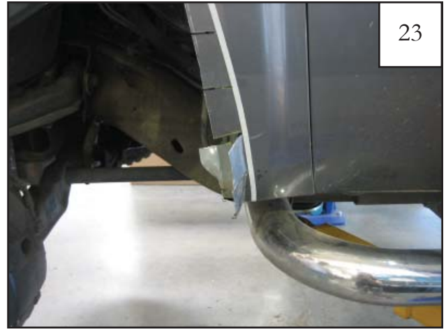
Bend lowest two metal tabs outward.
