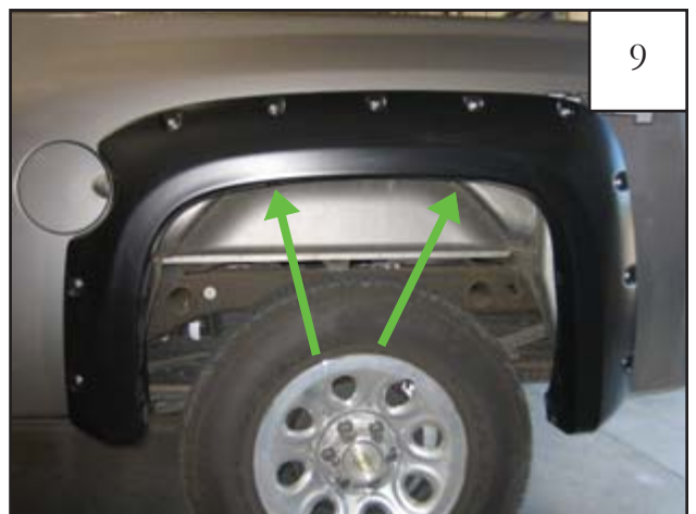
Reposition flare on fender. Start a supplied Screw (SW1-0058) through upper two hole locations and through each Clip (CL1-0022) installed in step 7. If needed, use awl to locate holes.
