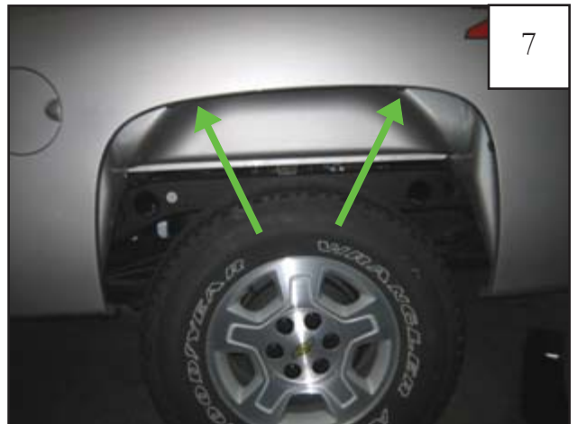
Slide a supplied Clip (CL1-0022) over top two factory holes. Clips may need to be adjusted to align with holes in flare. Note: Some vehicles with inner splash shield will need to remove factory fasteners in indicated locations before installing the clips.
