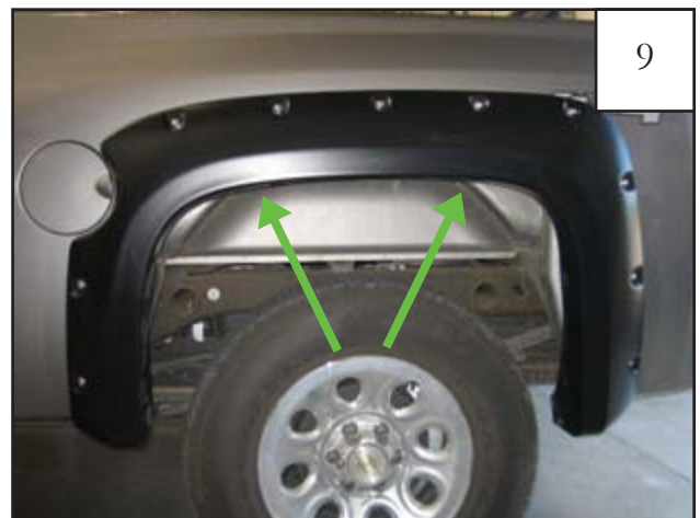
Reposition flare on fender. Start a supplied Screw (SW1-0058) through upper two hole locations and through each Clip (CL1-0022) installed in step 7. If needed, use scratch awl to locate holes.
