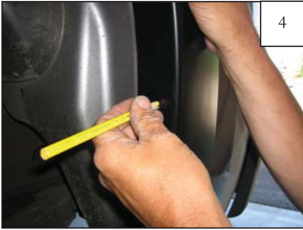
Holding flare in position on fender, use a grease pencil to mark seven hole locations.
