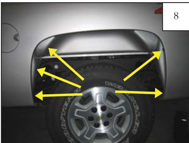
Slide a supplied Clip (CL1-0005) over lower five tabs. Clips may need to be adjusted to align with holes in flare.
