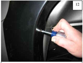
Start a supplied Serrated Flange Screw through each of the remaining holes and into each "S" Clip installed in Step 10.
