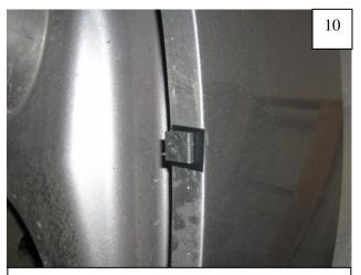
Slide a supplied "S" Clip over each black tab. Clips may need to be adjusted to align with holes in flare.
