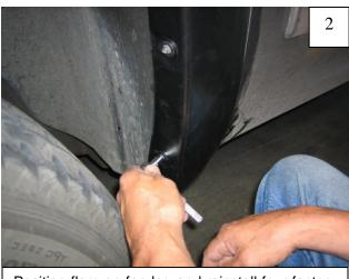
Position flare on fender, and reinstall four factory screws removed in Step 1.
