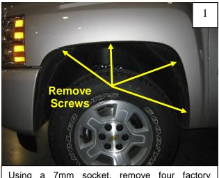
Using a 7mm socket, remove four factory screws. Retain screws for later use.
