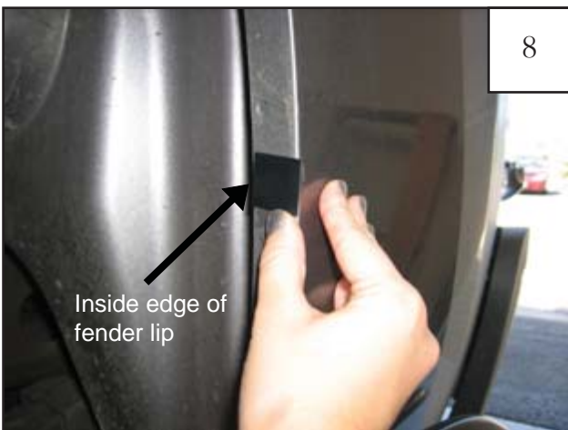
Center a supplied Tab (MT1-0002) over the six remaining marks made in Step 4, aligning edge of Tab with inside edge of fender lip (Tab may extend over outside of fender).
