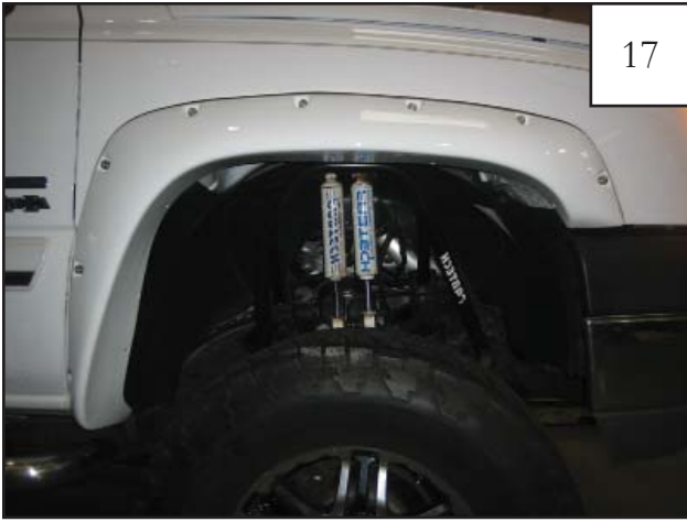
Completed front flare installation.
