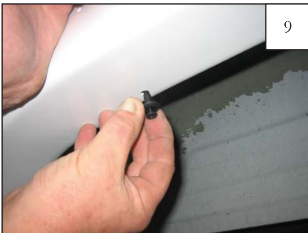
Position flare using supplied Retainers (RV1-P001) through factory holes. Do not fully fasten as flare will be removed after marking for drilling.
