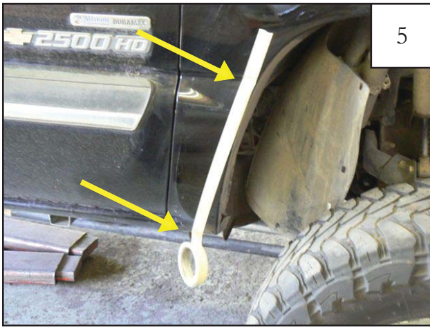
Run a piece of masking tape vertically from 0" at body line to 1.25" mark made in previous step.
