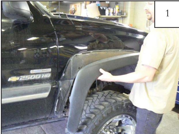
Remove factory flare using a flat blade screwdriver to pry up the head.
