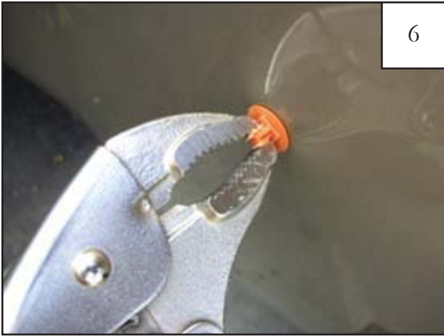
Remove two clips from front using vise grips, pulling with a rocking motion. See step 7.
