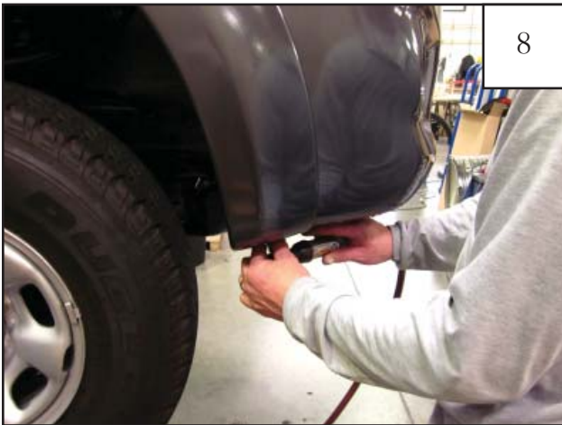
Remove 3 factory screws from under front bumper. Set aside for reinstallation.
