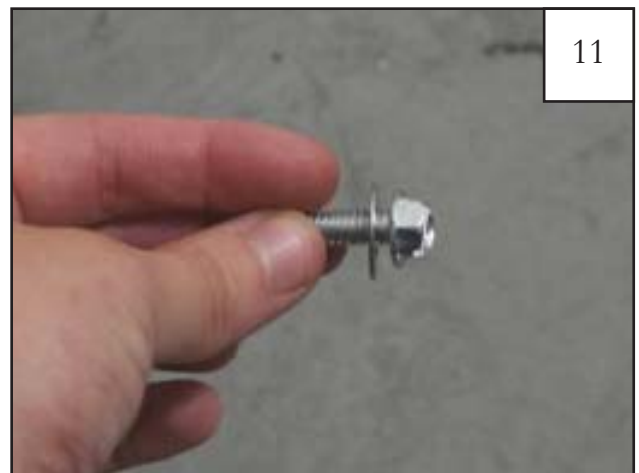
Slide a supplied Washer (WA1-0015) onto a supplied Hexhead Slot Screw (SW1-0005)
