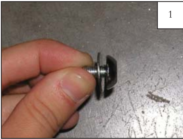
Put a Washer (WA1-0012) on each Bolt (SW1-0059).
