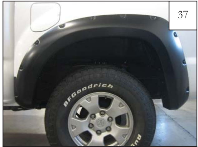
Completed rear flare installation.
