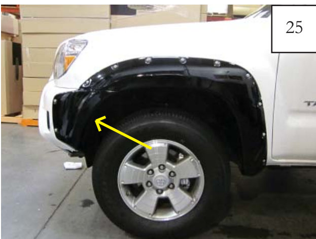
Make sure bumper piece is aligned with the style line. Install supplied 20mm hex screw (SW1-0036) into factory hole on front bumper and tighten
