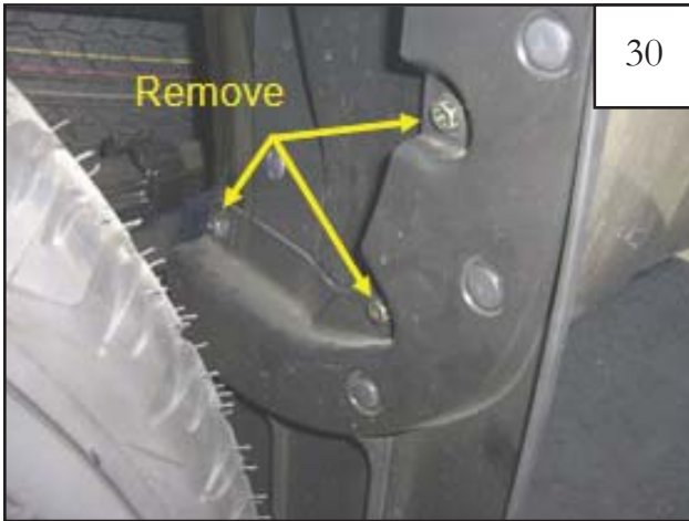
Remove three factory screws from mud flap. Discard mud flap.
