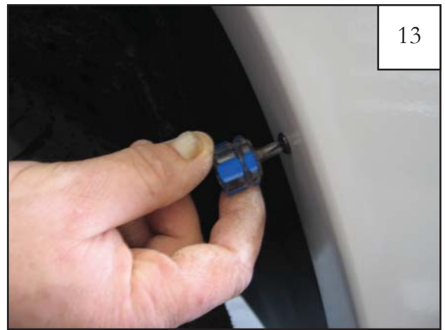
Start supplied serrated-flange screws through holes in flare and into the "S" clips installed in step 11. Note: Do not tighten screws until door piece is installed.
