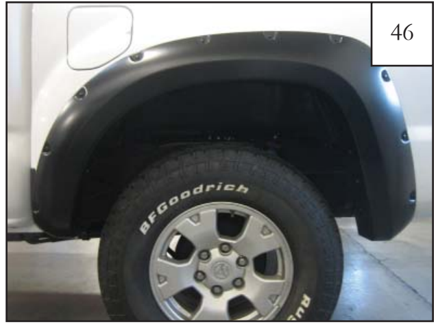
Completed rear flare installation.
