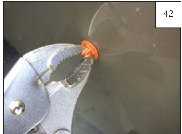
Remove three clips from fender using vise grips, pulling with a rocking motion. See step 43.
