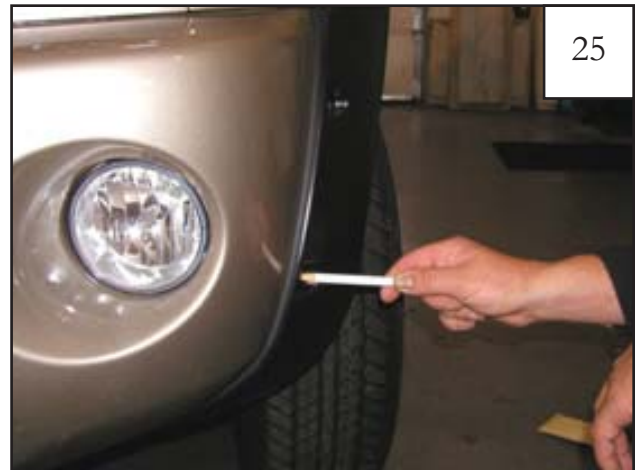
Using a grease pencil, mark hole locations for Front Bumper Piece pockets. 2 places.
