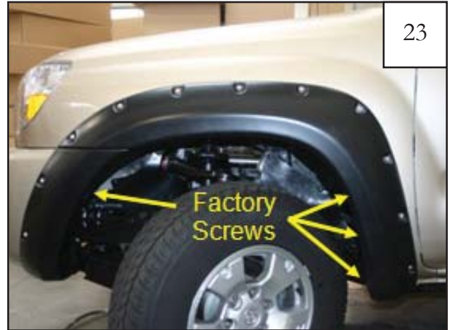
Reposition flare on fender and install four factory fasteners through holes in flare and into factory holes.
