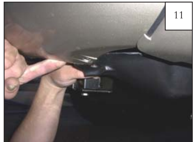
Pull down bumper cover and splash shield.
