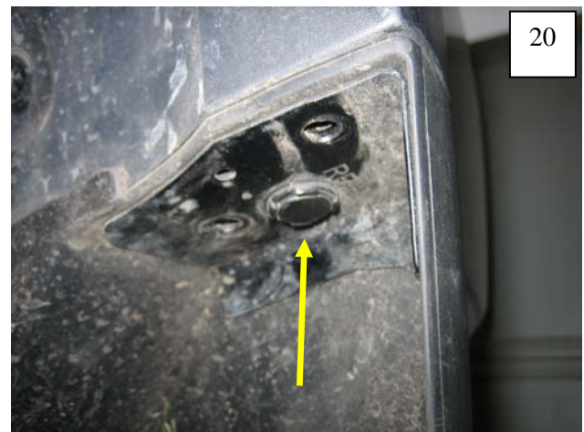
Remove one plastic fastener from mud guard.
