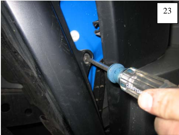
Remove bolt located behind rear plastic panel. NOTE: if the socket does not fit in the enclosed space, a Phillips screwdriver will work.
