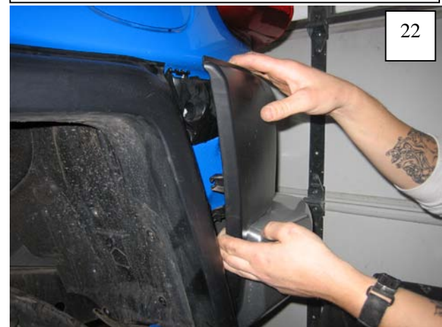
Pull back rear plastic panel to access bolt inside. Plastic clips will release, making a popping sound.
