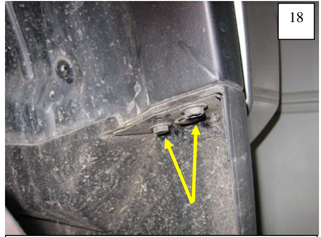
Remove two bolts from mud flap.
