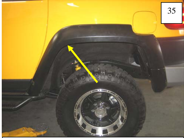
Install one supplied Christmas Tree Fastener in top forward hole. Check that edge trim is seated correctly, then tighten all bolts.
