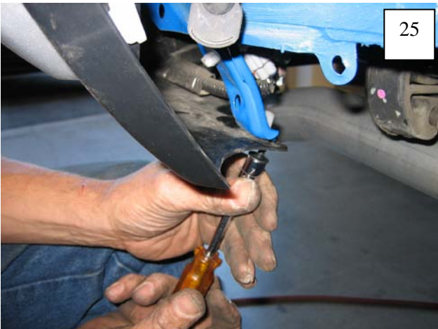
Remove bolt from underside of factory flare (behind panel). Pry flare from fender, releasing plastic clips.
