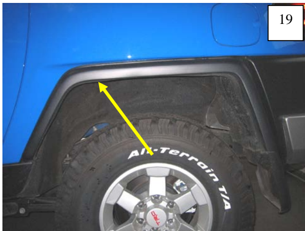
Using a pry tool or flat head screwdriver, remove one plastic fastener.
