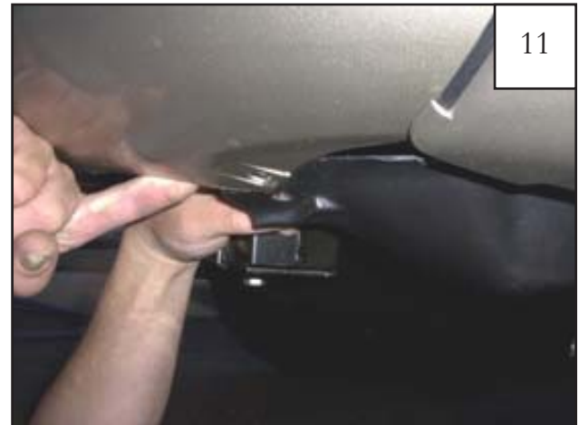
Pull down bumper cover and splash shield.
