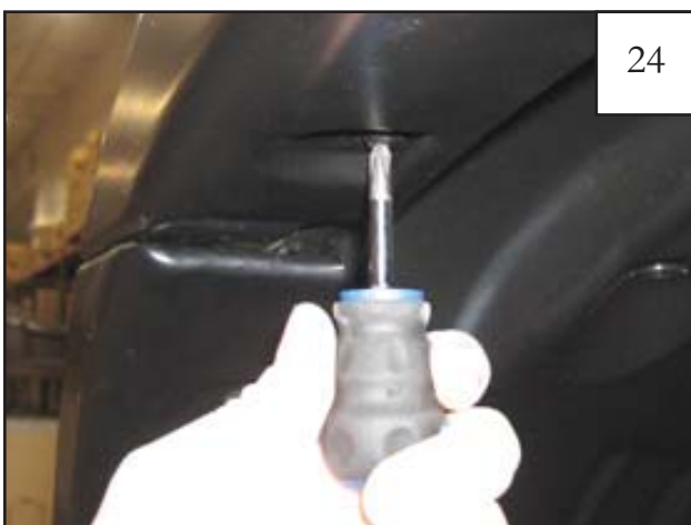
Install a supplied Screw (SW1-0050) through hole in flare and into Clip installed in step 22. 4 places.
