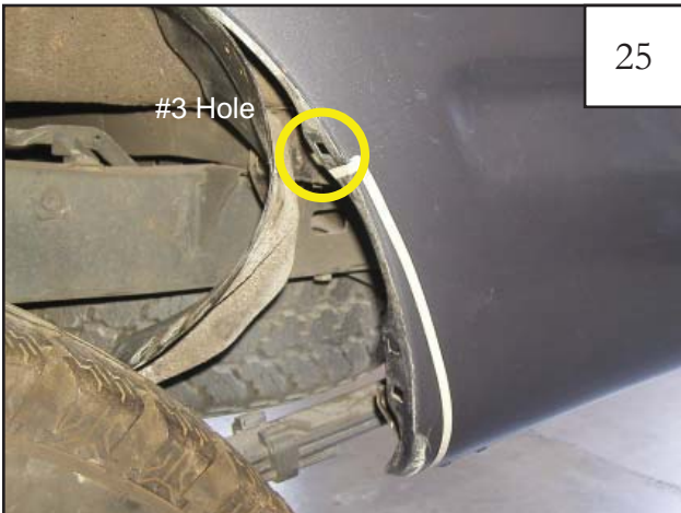
REAR - Using the 3rd hole up from the bottom as a guide, make a tape line along lower edge of hole horizontally.
