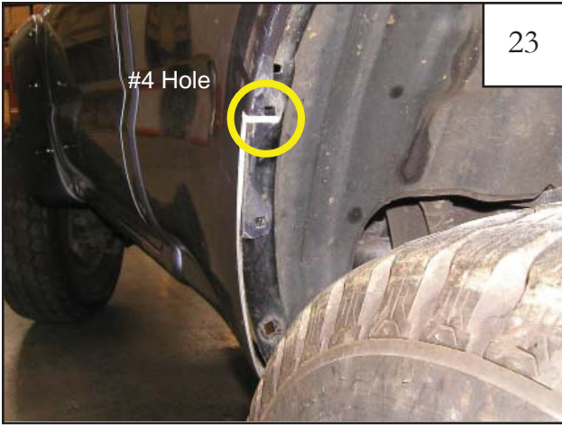
FRONT - Using the 4th hole up from the bottom as a guide, make a tape line along lower edge of hole horizontally.
