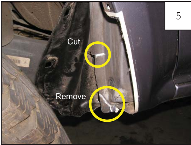
Cut fire wall weld seam in areas shown.
