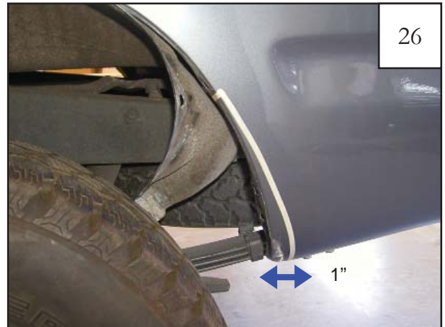
Measure out 1" at bottom of rocker. Make a tape line from bottom of rocker up, intersecting the first tape line. Using a reciprocating saw, cut fender on the inner edge of tape line.
