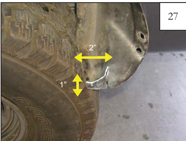
Trim REAR splash shield as shown for optimum clearance. Measure up 1" from bottom and 2" in, intersecting the two lines.
