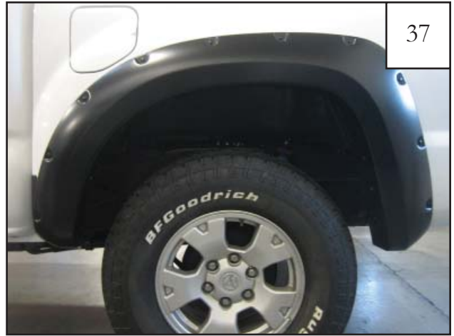
Completed rear flare installation.
