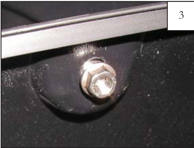
FRONT MAIN & REAR FLARE ONLY: Place a Nut (NU1-0019) over the end of each Bolt and tighten, using a 1/2" wrench for the Nut and the supplied Torx Bit (SW1-0052) for the Bolt. Repeat for remaining pockets.
