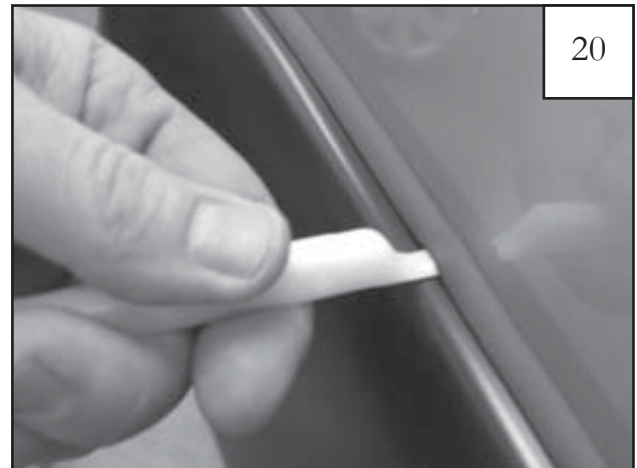
Using flat end of supplied Edge Trim Tool, seat edge trim against flare by inserting straight end between edge trim and flare at one end. Next, slide around entire edge to the other end.
