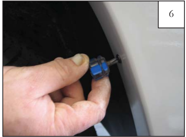
Start supplied serrated-flange screws through holes in flare and into the "S" clips installed in step 4. Note: Do not tighten screws until door piece is installed.
