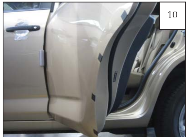
Remove door piece from door. Center a supplied black tab over each mark made in step 8.
