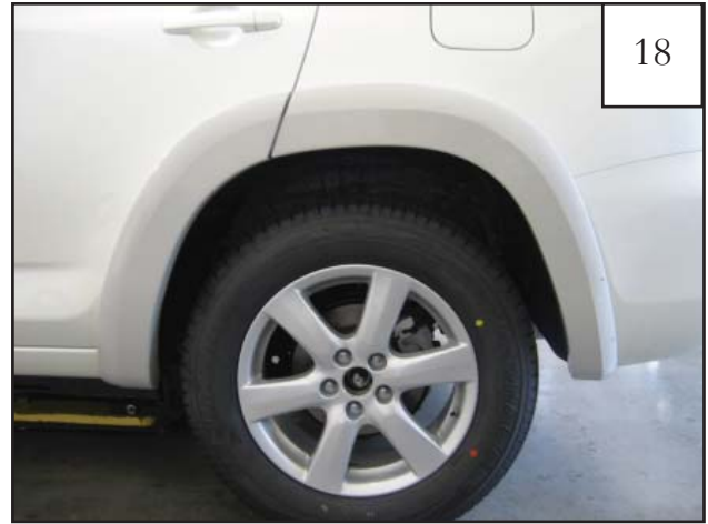
Close vehicle door and check alignment of door piece to rear main flare. Adjust rear main flare for proper alignment. Once satisfied, tighten all rear main flare screws using a right angle #2 Phillips stubby screwdriver
