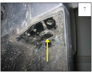
Remove one plastic fastener from mud guard.
