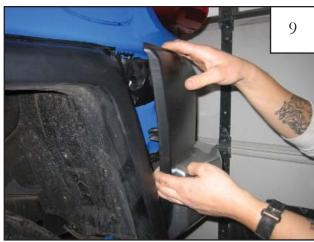
Pull back rear plastic panel to access bolt inside. Plastic clips will release, making a popping sound.
