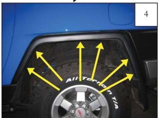
Using a 10mm socket, remove six bolts.
