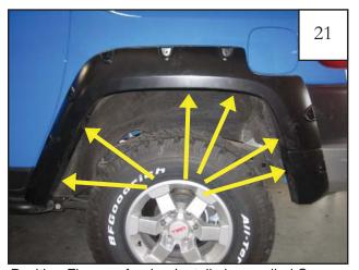
Position Flare on fender. Install six supplied Screws (SW1-0036). Do not tighten. NOTE: It is helpful to install one of the top Screws first.
