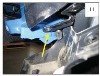
Remove 10mm bolt to remove mud flap completely.
