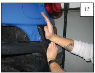
Using a pushing motion to engage clips, replace rear plastic panel.
