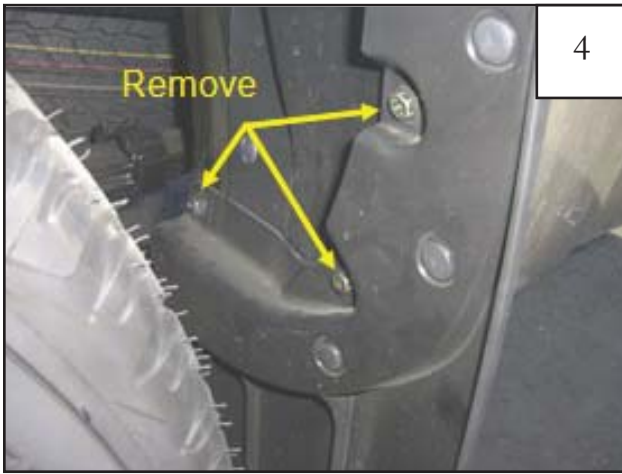
Remove three factory screws from mud flap. Save screws for reinstallation. Discard mud flap.
