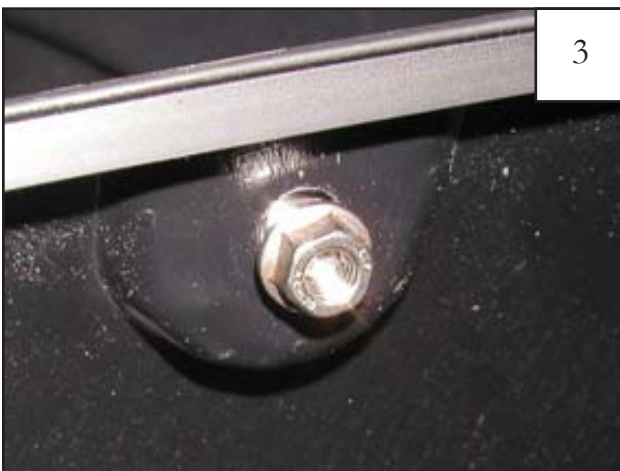
Place a Nut (NU1-0010) over the end of each Bolt and tighten, using a 1/2" wrench for the Nut and the supplied Torx Bit (SW1-0022) for the Bolt. Repeat for remaining pockets.
