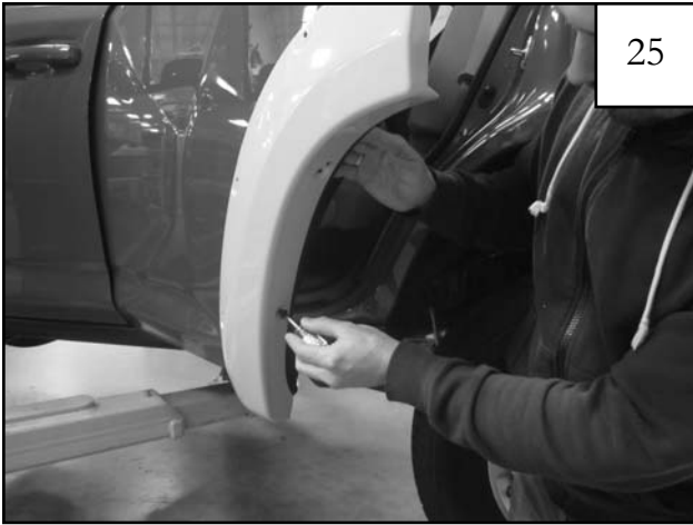
Install supplied Truss Head Screws (SW1-0044) into holes. Screws are attached to factory flare. DO NOT OVER TIGHTEN SCREWS.
