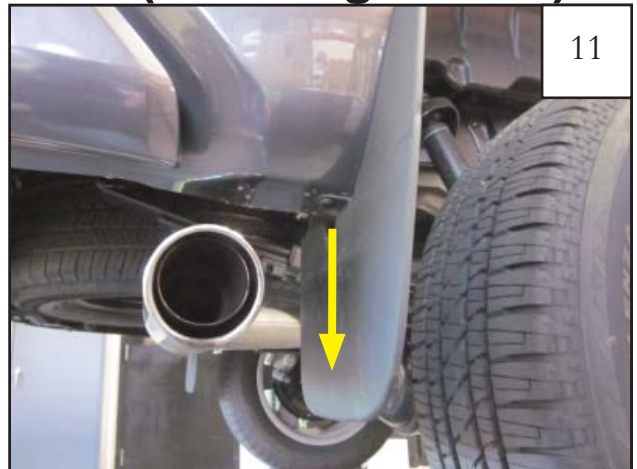
Remove push retainer from underside of factory mud guard.
