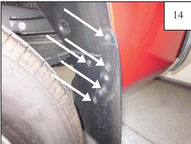
Remove five hex bolts from factory mud flap using a 10mm socket.
