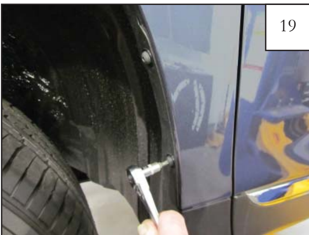
Using a 3 mm Allen Wrench, remove two factory screws from rear of wheel well. Save for reinstallation.
