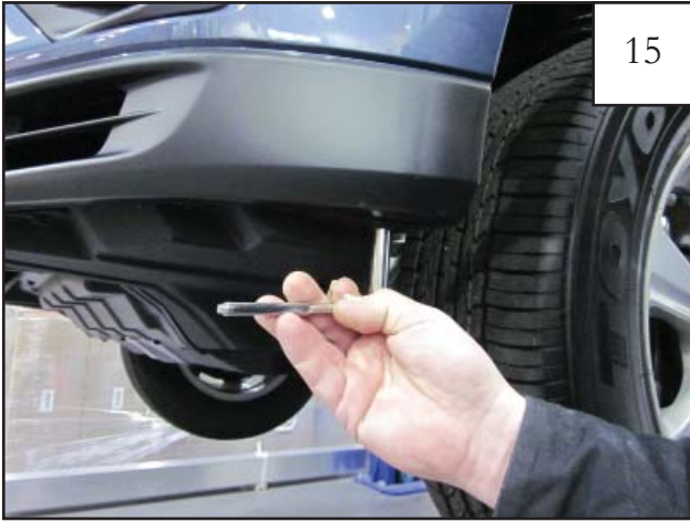
Using a 10mm socket wrench, remove factory bolt at front underside of wheel well. Save for reinstallation.
