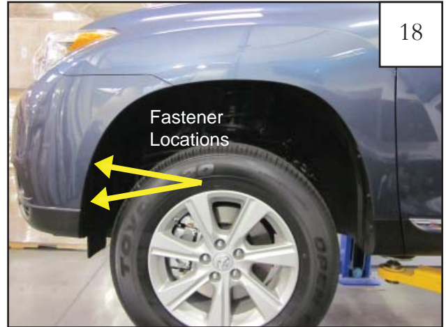
Factory fastener locations.
