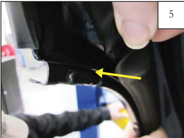
Pull gasket up to expose edge of door. Align Inner Door Piece Indexing Bump with edge of door.
