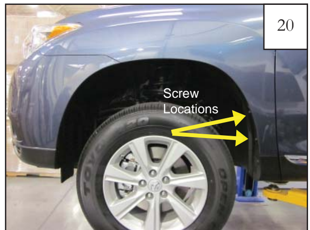
Two factory screw locations.
