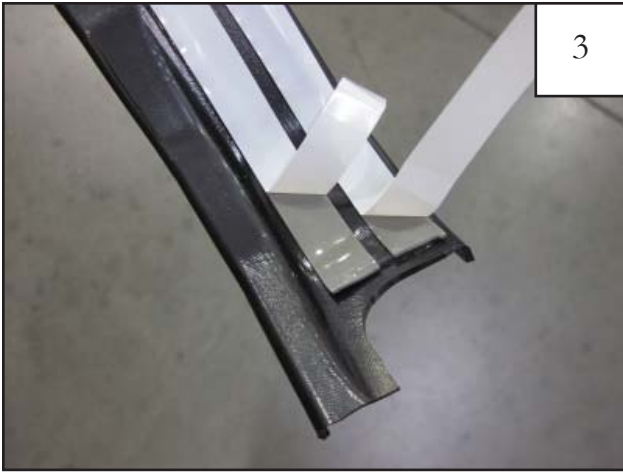
Start to peel white vinyl liner from tape at bottom of Inner Door Piece, folding tabs toward the outer curvature of the part and ensuring that inner liner is behind the outer liner.
