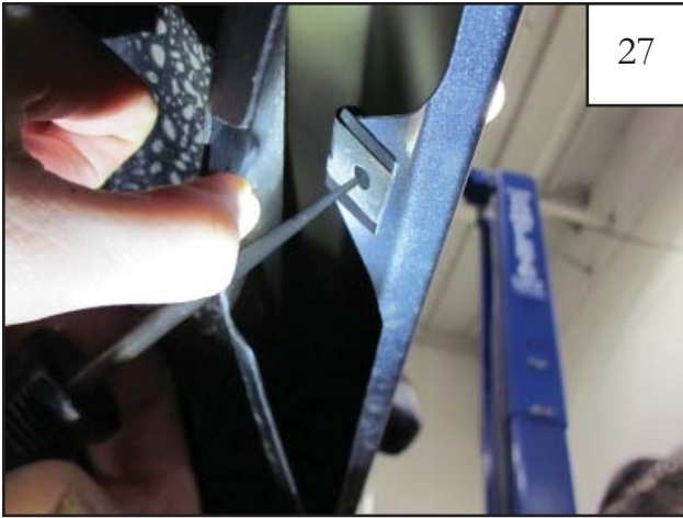
Using awl to poke hole through Tab using Clip installed in Step 26 as a guide. With Clip installed, tuck liner back in. Two locations
