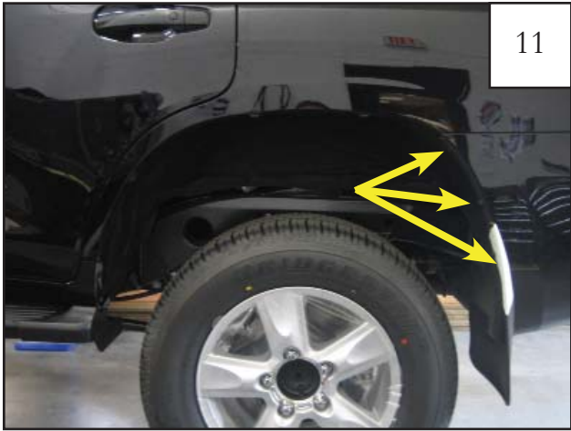
Using a socket with a T30 Torx bit, remove three factory screws. Discard.
