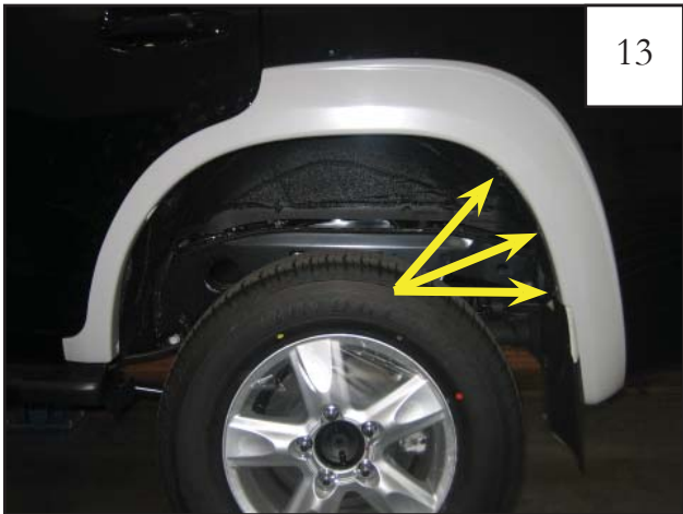
Position Rear Main Flare on fender, and hand start three supplied Hex Screws in rear of rear wheel well, starting with the top screw and working your way down.
