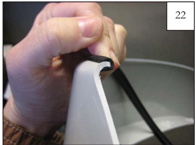
Install Edge Trim on Door Piece. Refer to Edge Trim Installation section for instructions.
