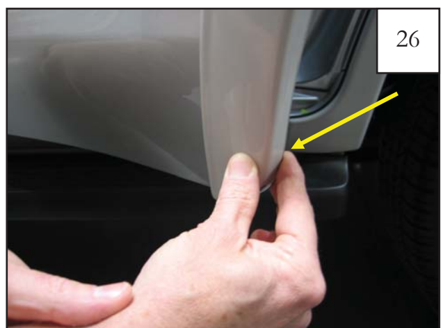
Align lower curve of Door Piece flush with lower door edge.
