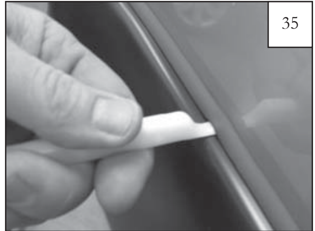
Using flat end of supplied Edge Trim Tool (ET1-0001), seat edge trim against flare by inserting straight end between edge trim and flare at one end. Next, slide around entire edge to the other end.
