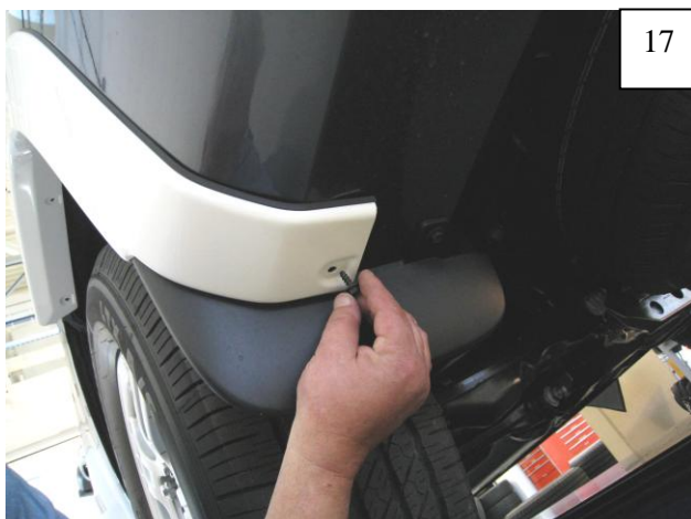
Hand start a supplied Hex bolt in underside of Rear Main Flare at mud flap area. Do not tighten.
