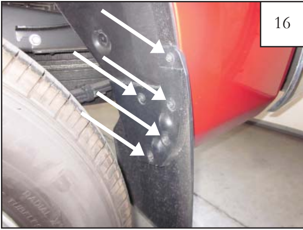
Remove five hex bolts from factory mud flap using a 10mm socket.
