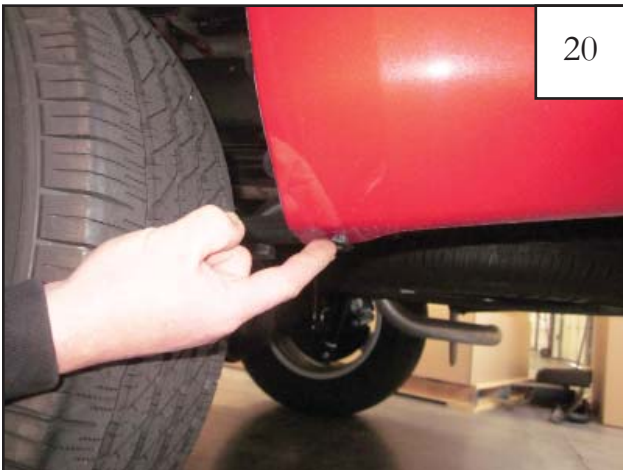
NOTE: If the lower rear wheel well does not contain a plastic grommet, insert supplied Grommet (GR1-0001) into the factory hole as shown.
